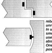
**DOUBLE LEAFED DOORS** In order to provide equal resistance to fire from either side, two seals are recommended for rebated meeting stiles and unrebated meeting stiles. In unrebated stiles a cold smoke seal on one stile only is used to compensate for absence of rebate. One seal only required at heel position.
