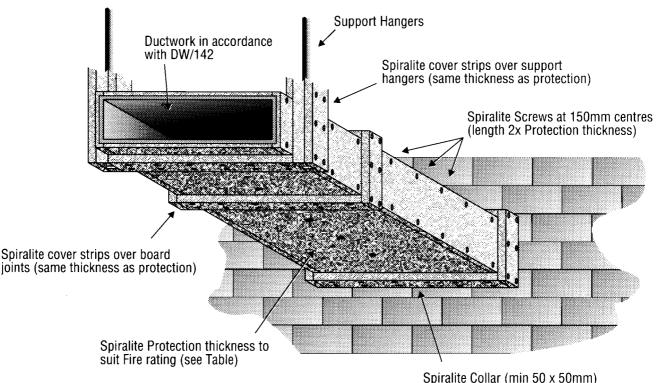
Spiralite Collar (min 50 x 50mm) glued to wall using Spiralite Adhesive
