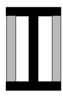
FIXING SEODENCE mm wide noggings flush with flange toes, at 1800mm centres
