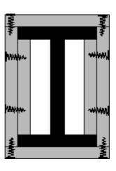
C. Cut flange panels to width of section, plus 2 x nominal protection thickness. Secure both edges onto web panels using Spiralite Screws at 150mm maximum centres.
