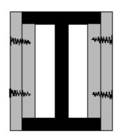
B. Cut web panels equal to depth of section and secure on noggings with Spiralite screws at 200mm maximum centres
