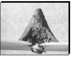
In a fire situation, the cover expands internally to fill the available space with fireresistant insulating material.
