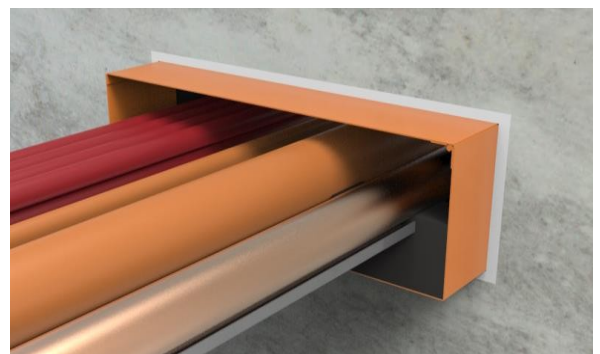
Sealant to all annular gaps around the box
